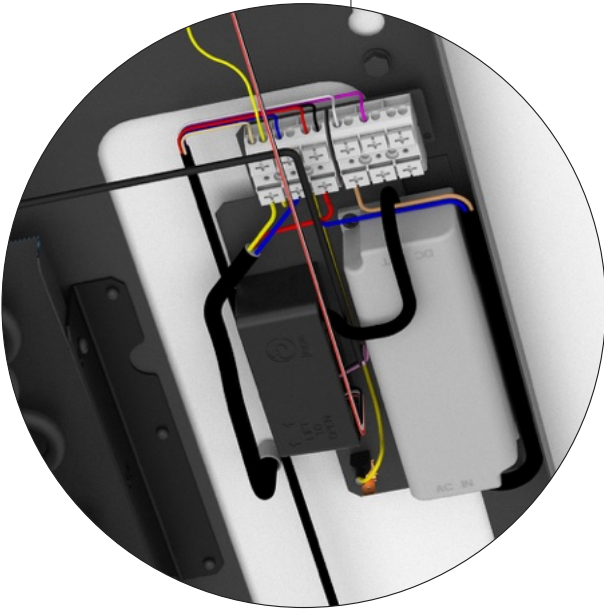
CONDENSING COOLING 230 VAC CONNECTION WITH WATERTIGHT POWER SUPPLY AND PRE-ASSEMBLED CONDENSATE PUMP WITH BREAKER POINT (CLASS I DEVICE)
